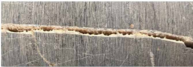
Partly open natural fracture in core
